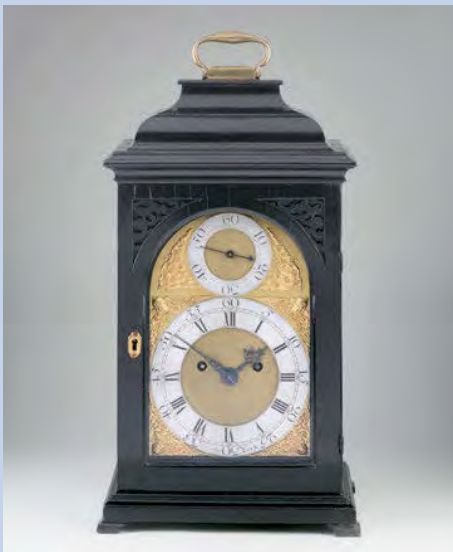
HENRY HINDLEY, YORK A rare ebonised striking table clock with large seconds dial and pull quarter repeat. Circa 1750
