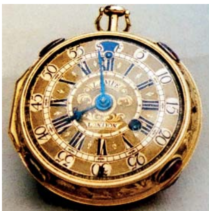
An automata watch by Lampe, London, with figures of Adam and Eve in white on a gilt background, verge escapement, the case embossed with Oriental and mythological scenes
